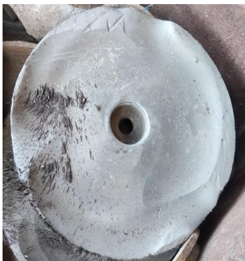
Figure 1. Appearance of a disc cast that has become unusable
